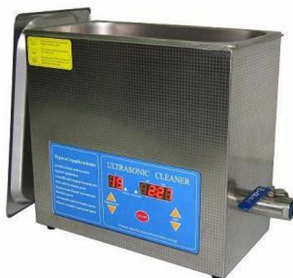
Figure 2.3 MTI Ultrasonic Bath Sonicator of 40 KHz [20]
