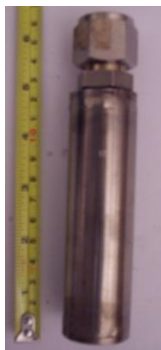
Figure 2.5 Stainless Steel Autoclave Used for Solvothermal Synthesis
