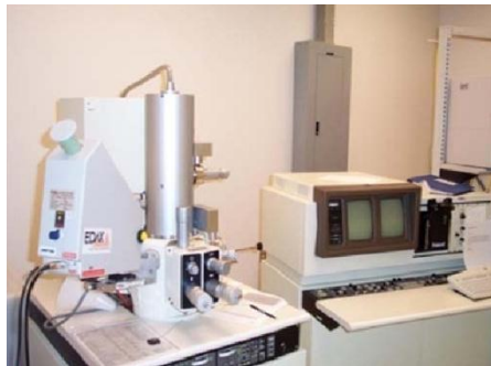
Figure 2.10 Hitachi S800 SEM Used for Surface Analysis [24]
